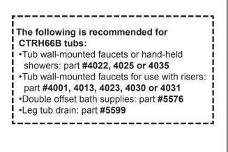
Gallon Capacity: Shipping Weight: Empty Weight: Filled Weight: 42 540 lbs. 360 lbs. 711 lbs. Cat. No. CTRH66B-WH
